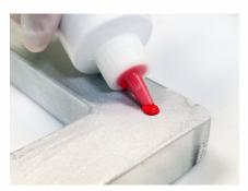
DYNABOND Two-Part Frame Adhesive used to precoat frame
