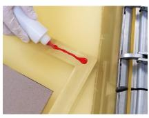
DYNABOND Two-Part Frame Adhesive used after stretching
