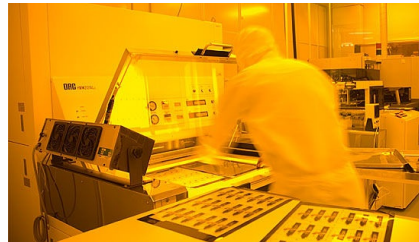
Cleanroom Exceeding Class 10,000 (ISO 7) Standards
